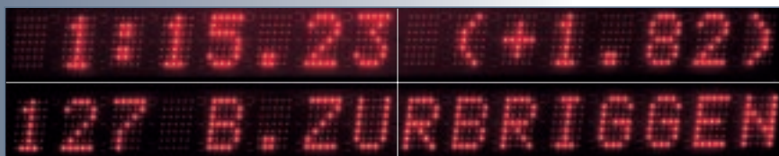
Four HL 980 displays with competitor's time and gap compared to the best time, number and competitor's name.
